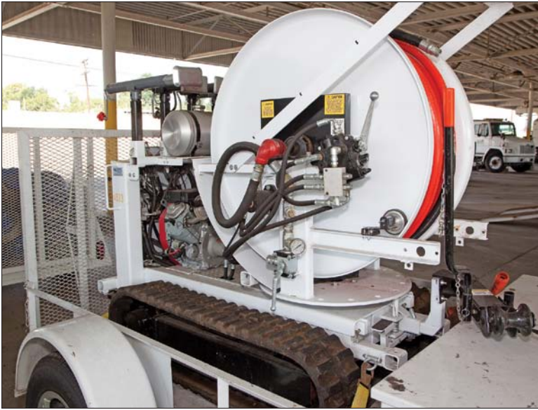
A Prowler easement machine from 3T Equipment helps the Glendale crew reach off-road locations for cleaning and inspection.
