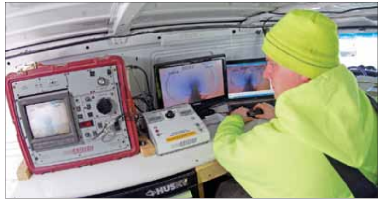
Left photo: Kyle (left) and John Baxter prepare to launch an Aries Pathfinder camera. Right: Kyle monitors an inspection inside the company's camera van from Aries Industries Inc. Equipment includes a Saturn III control unit, a tractor control unit and a laptop computer and auxiliary monitor.
