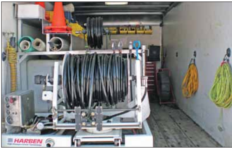
A powerful waterjetter forms the heart of Advanced Hydro-Jet's box truck. The truck also carries a CIPP lining system and other equipment.
