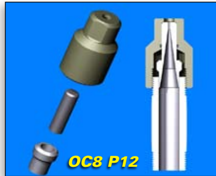
The OC8 P12 Holder and OC Carbide Inserts for 15K psi, 3/4" npt, female connection.
