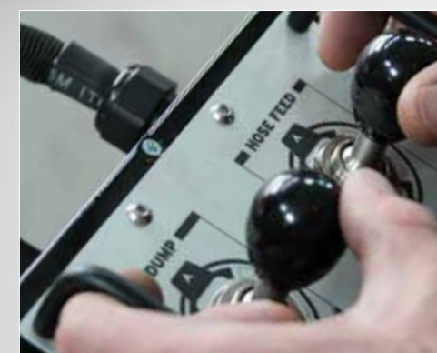
TETHERED REMOTE Allows freedom of movement outside the blast zone for safety and visibility.
