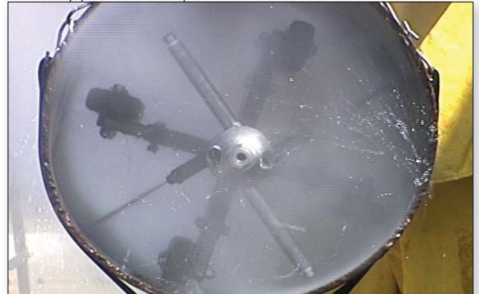
BJV-20k w/ nipple extensions & BJ-288 Centralizer.
