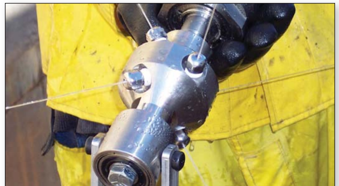
BJV-20k nozzle with optional HC 090 pull ring.
