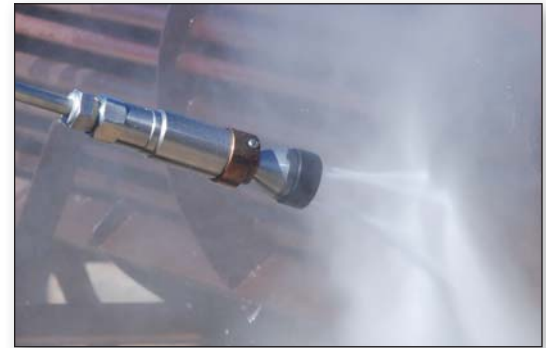
A 4-jet configuration at work on a tube bundle.
