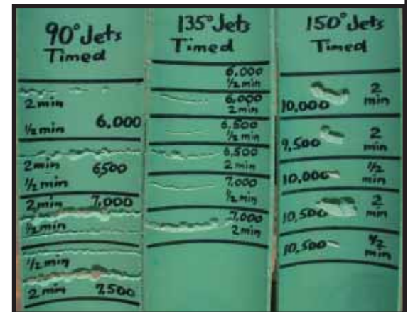
Contact time at pressures above the damage threshold is important
