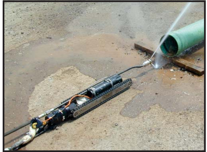
Zoom Sewer & Drain develops crawler/root cutter
