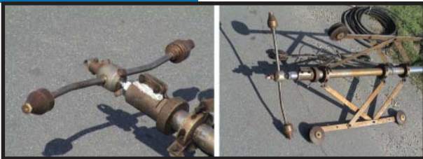
RJV, BJ 186-M-P12 Centralizer, and Gun Nozzles
