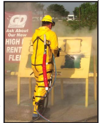
Gardner-Denver demonstrates 40 Kpsi self-rotating Barracuda
