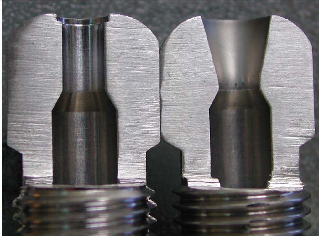
Figure 7. Steel nozzle on the right showing abrasive erosion from very dirty water
