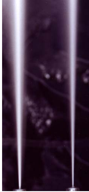
Figure 2. Jet pattern produced by the 5% binder nozzle after 15 hours on the left, compared to new of the same material and design on the right
