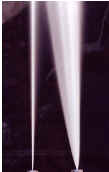
Figure 3. Jet pattern produced by the 15% binder nozzle after 40 hours on the right, compared to new of same design and material on the left
