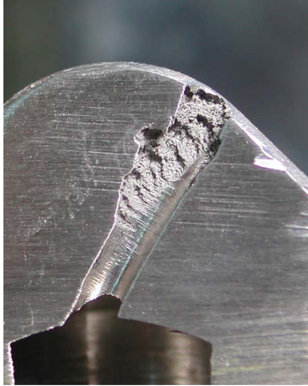
Figure 8. Steel nozzle with cavitation erosion
